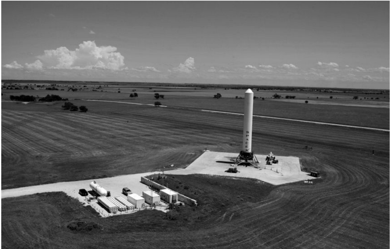
SpaceX tests new engines and crafts at a site in McGregor, Texas. Here the company is testing a reusable rocket, code-named “Grasshopper,” that can land itself. Photograph courtesy of SpaceX
